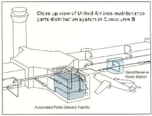
The new 10" CTS parts delivery system allows the sidnes to perform more alreraft maintenance within a shorter period of time. This system minimizes the time that aircraft are parked at the gate, saving both time and money.
